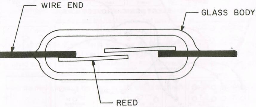
When no magnets nearby the reeds are not touching, so electricity cannot pass through. This is similar to an open switch. When a strong magnet is brought near the Switch, the reeds pass the magnetic lines of force and become attracted to each other like little magnets. This is then a closed switch. When the magnet is removed the reeds come apart because they are very soft iron which does not retain much permanent magnetism.
