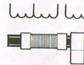
**ANTENNA COIL:** You'll use this part in radio circuits. It's a coil of wire wrapped around a dark colored rod made of ferrite, a special form of powdered iron.
