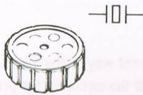
**PIEZO BUZZER:** The Piezo Buzzer in your kit will sound whenever electricity flows through it.
