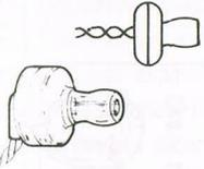
**MOTOR:** The Motor Assembly is one of the most interesting items included in your kit. It can be used either as an electric motor, or as a generator of electricity. In some of the projects you put the Fan on the Shaft of this motor/generator.
