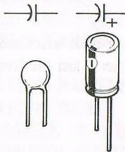
**CAPACITORS:** Capacitors store and release electricity as a circuit needs it.
