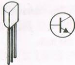
**TRANSISTOR:** Transistors have three connections instead of two like the other parts you have seen. You'll see why this is important later. In your kit, transistors act either as switches to turn things on and off or as amplifiers to make signals louder or to increase the rate of signal change, or frequency.
