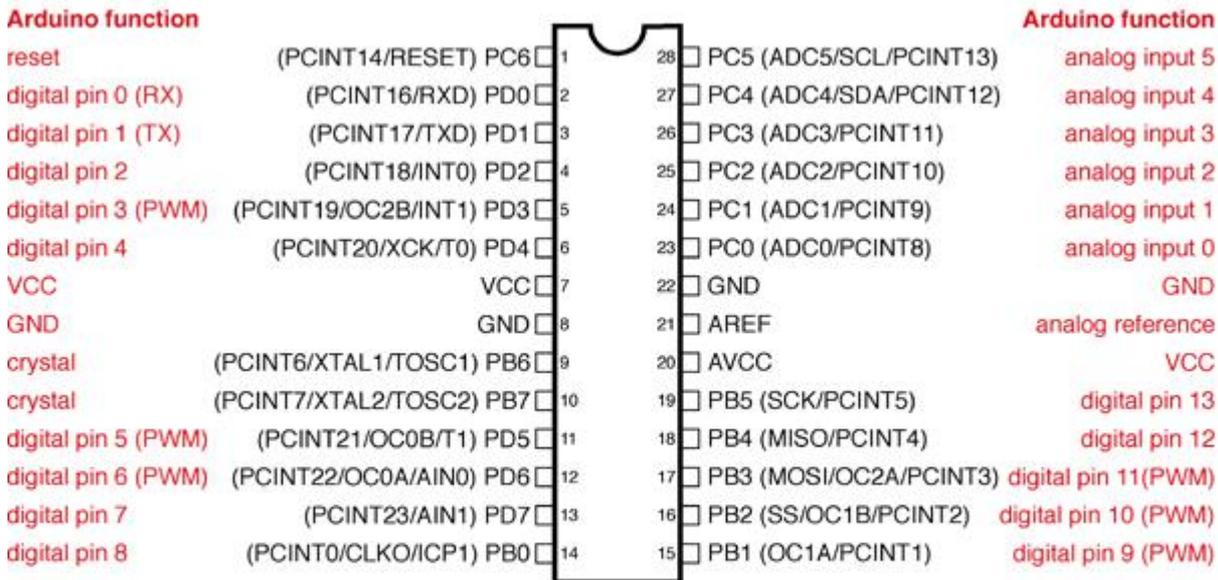
Digital Pins 11, 12 & 13 are used by the ICSP header for MOSI, MISO, SCK connections (Atmega168 pins 17, 18 & 19). Avoid low-impedance loads on these pins when using the ICSP header.
