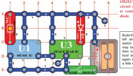
**OBJECTIVE:** To build a circuit that uses your voice to control a light emitting
