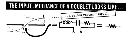
The radiation resistance is not an actual resistance. It is an equivalent resistance which, if connected in place of the antenna, would dissipate the same amount of power as the antenna radiates into space.
