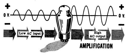
Because of your work with rectifier and power supply circuits, you now know all you need to know about rectification and the diode tubes that are used to do this job. Now you are ready to learn about the second main job a vacuum tube can do—amplification. In this section you will learn about the vacuum tubes that do the job of amplifying small AC voltages into large AC voltages.
