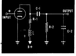
When the grid voltage swings negative, as at (b), the plate current decreases and the back emf across L is in the opposite direction. This then adds to the plate voltage—normally high anyway—causing another peak to appear at (b). Because of the effect of this inductance, it is always referred to as a peaking coil."
