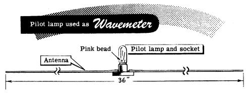
First, the transmitter is retuned until the bulb is brightest. Then, the intensity of the radiation around the antenna is demonstrated by moving the dipole, parallel to the antenna, from the center out to either end. Observe that the bulb is brightest when the center of the wavemeter dipole is lined up with the center of the antenna, and the bulb goes out when the center of the wavemeter dipole is in line with the end of the transmitting antenna.
