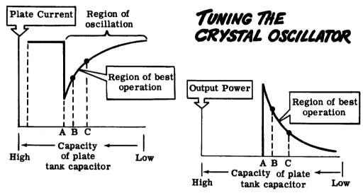
Since a crystal has low frictional losses, it doesn't require much feedback to sustain oscillations. Besides, a large amount of voltage across the crystal plates can make the crystal vibrate so hard as to overheat or shatter—much as a powerful explosion causes window panes to vibrate so strongly as to shatter. Overheating causes frequency drift. Thus, smaller feedback results in a greater safety factor and in less frequency drift.
