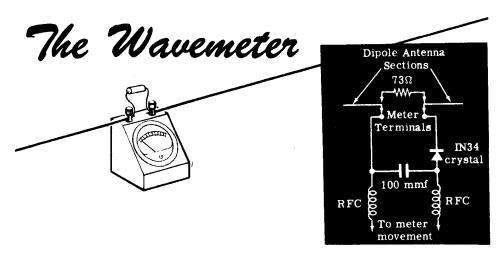
The instructor places the wavemeter far enough away from the transmitting antenna so that the meter needle does not deflect off scale. Then, the transmitter frequency is varied until the meter goes through a peak reading. At this point the transmitting antenna is exactly a half-wavelength long and is therefore radiating at maximum.
