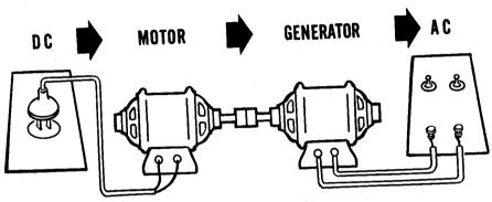
A dynamotor is a rotating DC machine that operates from a low voltage DC source and puts out one or several high voltage DC outputs. It is basically a DC motor and a DC generator built onto one armature and having two or more windings and two or more commutators. Dynamotors are usually operated from 6-, 12-, 24- or 32-volt storage batteries and deliver from 250 to over a thousand volts DC at various current ratings.
