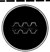
If the transmitter output shows breaks in the modulation pattern, the transmitter is said to be "over-modulated." This is usually due to excessive modulating voltage but may also be due to insufficient signal voltage on the grid or excessive grid bias voltage.
