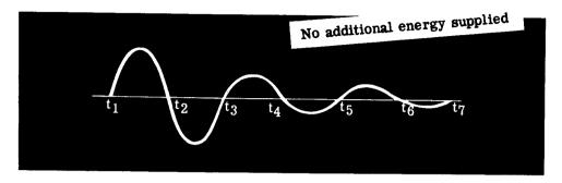
This is called a "damped" wave. It is like a sine wave, but with the height (amplitude) of successive cycles diminishing gradually. The time interval remains the same.
