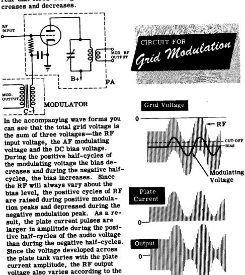
Grid modulation is used in compact or mobile transmitters because this type of modulation does not require a modulator with a large power output. When the modulator's weight is only a minor consideration, plate modulation with the larger modulator it requires is used because it produces much better results than grid modulation.
