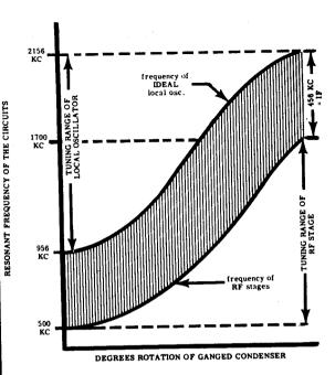
The first step is to adjust the trimmers on the two-ganged variable capacitor. Since these trimmers are in parallel with the tuning capacitors, they affect the total capacitance more at the high frequency end of the band (when the variable capacitor has minimum capacitance) than at the low frequency end. For this reason, the trimmers will be adjusted at 1500 kc, which is close to the high end of the broadcast band.
