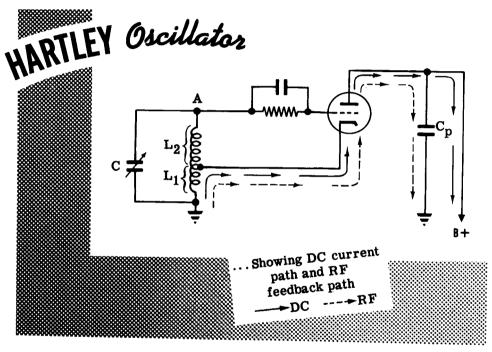
Once oscillation has begun, the cycle is very much the same as in the Armstrong oscillator. The tube is biased below cut-off from shortly after the top plate of the LC circuit, point A, has reached its peak positive value until shortly before it reaches its peak positive value again. During all this time the tube serves no purpose whatsoever, and the surge of electrons through the tank circuit goes on solely because of the flywheel effect of that LC circuit.
