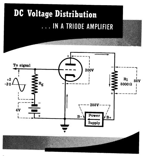
On the next sheet you will see how the load voltage and the plate voltage change when the signal is applied to the grid.
