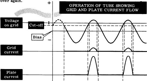
The tube, the grid resistor and capacitor and the power supply serve no purpose whatsoever during most of the cycle of oscillation. The LC circuit is the oscillator. All that these other components do is provide the means to give the LC circuit a voltage kick for a brief portion of the cycle. The "flywheel effect" keeps the electrons surging around the LC circuit with no other aid.
