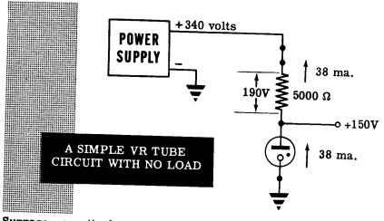
Suppose you attach an 8 ma. load to the 150 volt terminal. Of the 38 ma. flowing through the dropping resistor, 8 ma. flows through the load and 30 ma. flows through the VR tube. Since the VR tube current is yet within the rated range of 5 to 40 ma., the VR tube adjusts its internal resistance so that the plate voltage remains at 150 volts.
