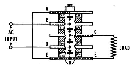
To get from the pictorial to the schematic diagram, just imagine the two end units being rotated around as shown below. Before you continue, make sure you understand the relationship between the physical unit and the schematic.
