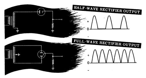
The electronic circuits which are connected to the power supply output cannot use a pulsating voltage of this sort. What these circuits require is a steady DC voltage with as little pulsation as possible. The purpose of the filter circuit is to remove the pulsations from the rectifier output and deliver a steady DC voltage.
