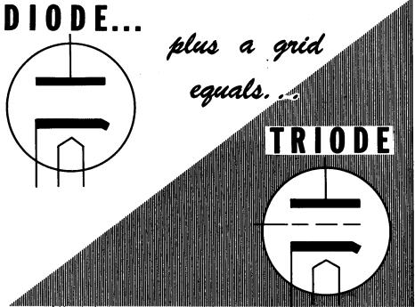
As in the diode, saturation in a triode occurs because there is a limit to the amount of current which the cathode can emit. In the triode, saturation (limiting current) can be reached at a lower value of plate voltage if a positive voltage is applied to the grid; in the diode, of course, it depends only on the plate voltage.
