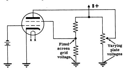
Notice that at high plate voltages above 300V, the plate current does not change when the plate voltage is increased. This is because the screen shields the plate from the space charge at the cathode which causes the screen to exert a greater control over plate current than the plate itself.
