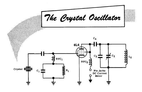
$C_3$  in parallel with  $C_2$  adds to its capacity and reduces the resonant frequency. This is required if the range of  $C_2L_2$  alone does not extend down to the crystal frequency.
