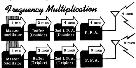
The reason that frequency multiplier circuits are used in transmitters is that an oscillator operates more satisfactorily at low frequencies. Therefore, if a high frequency is required, the oscillator operates at a low frequency and the multiplier circuits step up the oscillator frequency to the desired one.
