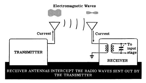
A receiving antenna should feed as much signal and as small an amount of undesired interference to the receiver as possible. It should be constructed so that the signal is not lost or dissipated before reaching the receiver. It should give maximum response for the frequency or band of frequencies to which the receiver is tuned. An antenna can also be directional, which means that it will give best response in the direction from which the operator wishes to receive.
