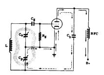
GRID LEAK BIAS—a method of bias in which excess electrons accumulate on the grid, producing a negative bias. They are allowed to leak off slowly through a large resistor which is placed in parallel with the grid capacitor or from grid to cathode. Making the resistor large enough produces more than cut-off bias and results in Class Coperation.
