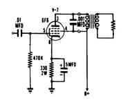
PHASE INVERTER — A circuit which uses one or two vacuum tubes to produce two signal voltages 180 degrees out of phase. It is also called a phase splitter and replaces the transformer in a push-pull circuit.
