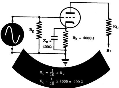
Since  $X_C = \frac{1}{2\pi f C}$ , the capacity of the bypass condenser can be found by using the formula  $C = \frac{1}{2\pi f X_C}$ , where f is the lowest frequency signal to be amplified. Suppose f is 60 cps and  $X_C$  is  $400\Omega$  as shown above, then C will be—  $\frac{1}{6.28 \times 60 \times 400} \approx 6.6 \text{ mfd.}$
