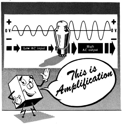
You will find that vacuum tubes are used to produce amplification in receivers, in transmitters, in sonar, in radar and in loran; and it is a foregone conclusion that when new types of electronic equipment come into use, some of the tubes there, too, will be used for amplification.
