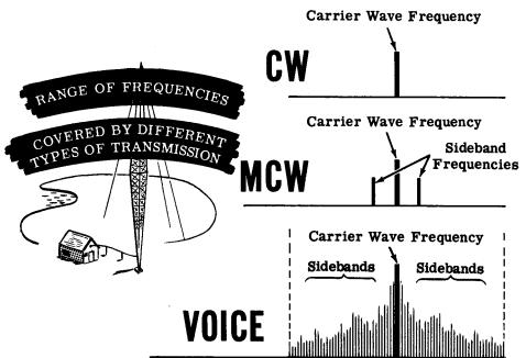
There are many different circuits which are used to obtain CW transmission. They look different and operate differently, but each has the same purpose—to turn the RF of the transmitter on and off. You will learn about some of these circuits on the next few sheets. In the next topic, you will find out more about MCW and voice transmission.
