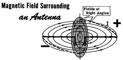
These electric and magnetic fields alternate about the antenna, building up, reaching a peak, collapsing, and building up again in the opposite direction, at the same frequency as the antenna current. In the process of building up and collapsing, a portion of these fields escape from the antenna and become the electromagnetic waves which radiate through space conveying the transmitted intelligence to distant receivers.
