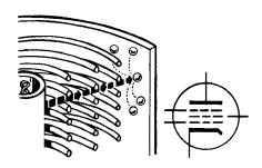
SINGLE-STAGE AMPLIFIER — A circuit consisting of a vacuum tube amplifier, biasing components, a load resistor, a decoupling network and a resistor and capacitor to provide coupling to another stage.
