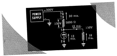
If the B+ voltage were to fall to 300 volts, the VR tube would have to adjust its internal resistance so that the plate voltage remains at 150V. Let's see if the tube can make this adjustment. The voltage across the dropping resistor is 300 volts - 150 volts = 150 volts. The current through the dropping resistor is:
