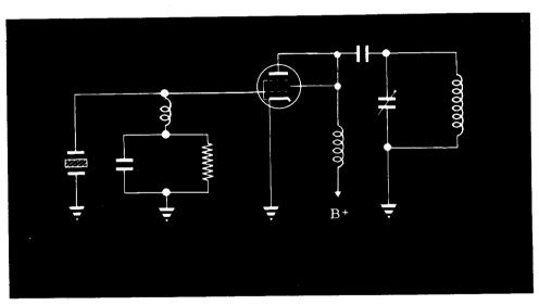
This circuit behaves like the TPTG oscillator in every respect. Feedback is obtained through the plate-grid capacity of the vacuum tube or by using a small feedback capacitor. This voltage feedback causes the crystal to vibrate mechanically at its natural frequency. When the crystal vibrates, an emf appears across the electrodes on the two faces of the crystal. This emf is applied to the grid. The changing emf on the grid controls the flow of plate current and hence the amount of feedback.
