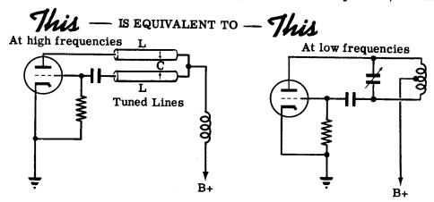
The characteristics of these tuned lines are calculated in the same way as characteristics of transmission lines, which you will find out about in "Transmitters." Inductance and capacitance of ordinary coils and capacitors is said to be "lumped." Inductance and capacitance of tuned lines is said to be "distributed." Here are some other high frequency oscillator circuits using distributed reactance (capacity and inductance).
