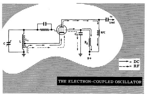
You can see that this is a modified Hartley oscillator. The modification consists in the replacement of the triode by a tetrode, which has an additional element, the screen grid.
