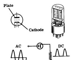
VACUUM-TUBE RECTIFIER CIR-CUIT — A diode vacuum tube connected in series with an AC voltage source to change AC to DC.
