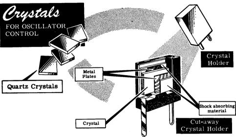
These crystals exhibit what is known as the piezoelectric effect. If a block of quartz is placed between two metal plates and pressure is applied, then a voltage difference will appear across those two plates. Also, if an AC voltage is applied across the two plates, the crystal will stretch and compress. Thus the crystal can convert mechanical pressure into electrical energy and electrical energy into mechanical vibration.
