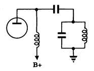
GROUNDING POINTS—Most oscillator circuits can be made to work with the plate, cathode or grid at RF ground potential.
