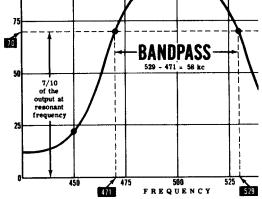
ALIGNMENT — The process of adjusting trimmers in a group of tuned amplifier stages so that all the stages tune to the same frequency. When a multiple-stage RF amplifier is correctly aligned, it will give more selectivity than a single-stage amplifier. When it is not correctly aligned, it may give far less selectivity or even tune to two frequencies at once.
