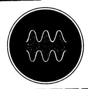
A pattern such as this would indicate that the positive peaks of the modulating voltage are not causing corresponding peaks in plate current. This may be due to improper grid bias, saturation due to low emission, or insufficient excitation of the power amplifier stage.
