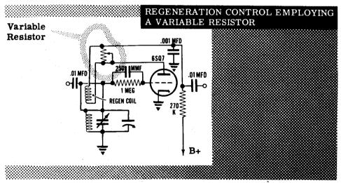
In the detector shown above, regeneration is controlled by a variable resistor placed across the tickler coil.
