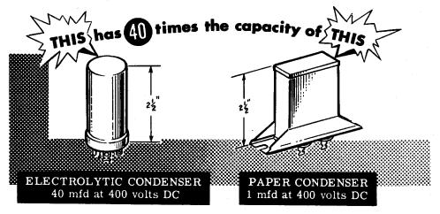
Power supplies rated at 600 volts or less usually use electrolytic filter condensers but when a higher voltage rating is required paper condensers are used. Electrolytics are polarized and failure to observe the correct polarity will not only permanently damage the condenser but may also cause it to break open and damage other parts.
