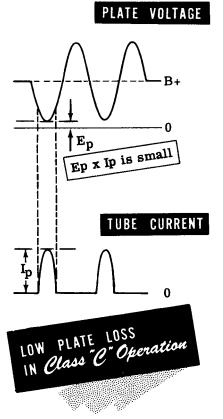
If the tuned circuit in the plate is not tuned to the frequency of the input signal, then the voltage across it will be lower—in proportion to how much it is mistuned. The further off it is tuned, the less power will appear across it and the more power will be dissipated by the tube itself. Then the efficiency of the amplifier is lower, the tube heats up more, and the power output is lower.
