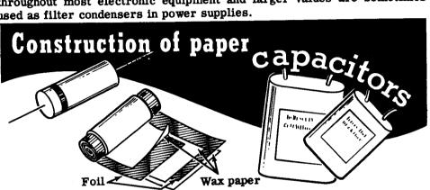
Paper condensers are not polarized and when operated within their voltage rating they last much longer than electrolytic condensers. However, large sizes of paper condensers are bulky and relatively expensive. They are normally not made larger than 16 mfd.
