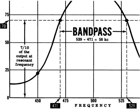
The output of the stage at the resonant frequency is 100 microvolts. Seventenths of this is 70 microvolts. The amplifier stage puts out 70 microvolts at 471 kc and at 529 kc. 529 kc minus 471 kc equals 58 kc. The bandpass of this particular RF amplifier is 58 kc. Now read the definition of bandpass again.
