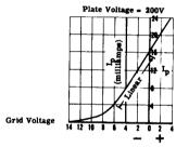
GRID BIAS — The amount of grid bias voltage determines the class of amplifier operation. In Class A the bias is less than cut off; in Class B bias is at or near cut-off; in Class C bias is much less than cut-off.
