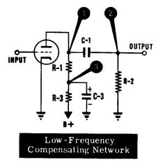
At (b), the current suddenly decreases and the voltage at point 1 rises as the condenser C-3 charges up. Thus between time (b) and time (c), the plate voltage is increasing.
