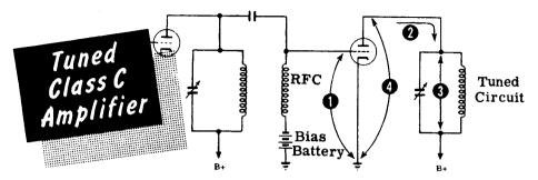
The operation of a Class C amplifier will become clear when you analyze what happens in a tuned amplifier such as the one shown in the schematic diagram. An AC signal is developed across the tuned circuit in the plate of the previous stage. This voltage also appears across the RF choke (RFC) in the grid circuit of the tuned Class C amplifier stage. The DC bias provided by the bias battery causes the tube to operate Class C.
