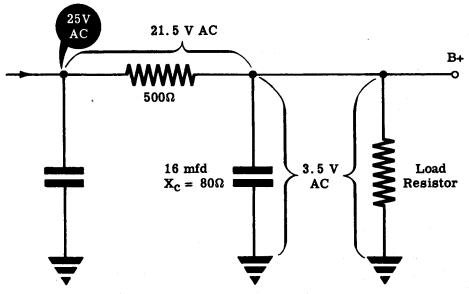
You see that the simple addition of a 500 ohm resistor and another filter condenser has succeeded in reducing the ripple voltage down to 3.5 volts which is about 1 percent of the total DC output. This amount of filtering is satisfactory for most applications in electronics.
