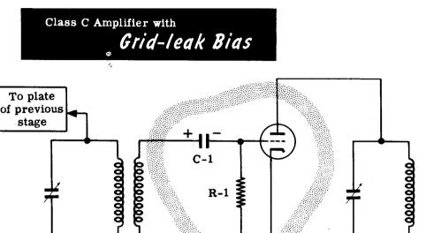
Whenever the signal drives the grid positive, the grid draws current and charges up capacitor C-1 to make the grid negative. Resistor R-1 provides a path for C-1 to discharge slightly between the pulses of grid current flow.
