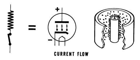
When the plate becomes the least bit negative with respect to the cathode, no electrons will flow from the cathode to the plate. The tube acts as if it were a resistor in series with a switch and the switch were opened up.
