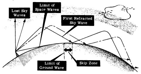
The critical frequency, which is the frequency above which no sky waves can return to earth, varies depending upon numerous factors such as the time of day, the time of year, the weather, etc. As a result, long distance communication can sometimes be achieved with frequencies which normally have no returning sky wave.
