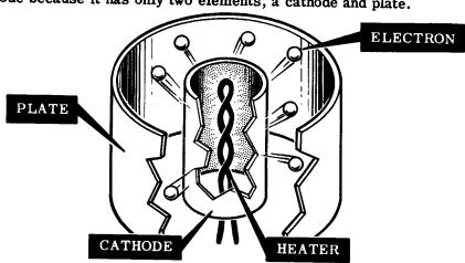
In addition to preventing the filament from burning, removing the air from the tube prevents the air molecules from interfering with the flow of electrons from cathode to plate. Sometimes the air is replaced by an inert gas which aids rather than opposes the electron flow.
