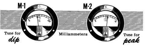
If the grid circuit has fixed bias or combination bias, no grid current will be drawn until the signal is fairly large. This will happen some time after the plate current meter has started to dip. For this reason, the rising grid current indication is sharper than the decreasing plate current indication.
