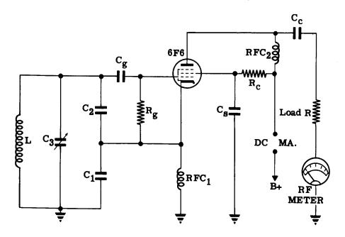
A pentode connected as a tetrode is used in place of the triode of the Colpitts oscillator. The cathode, control grid and screen, along with the tank circuit, act as a conventional Colpitts oscillator. The screen RF bypass capacitor,  $C_{\rm S}$ , shields this triode from the plate and supplies feedback across  $C_{\rm I}$ , the AC screen grid load.
