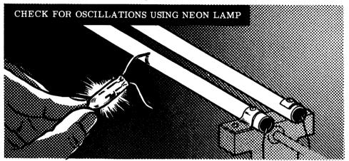
Once oscillations have been verified, the instructor demonstrates the presence of standing waves along the half-wave antenna by holding a fluorescent lamp close to and parallel with the antenna. The lamp is ignited by placing one end against the tuned line. The lamp glows at the ends and is out in the middle.
