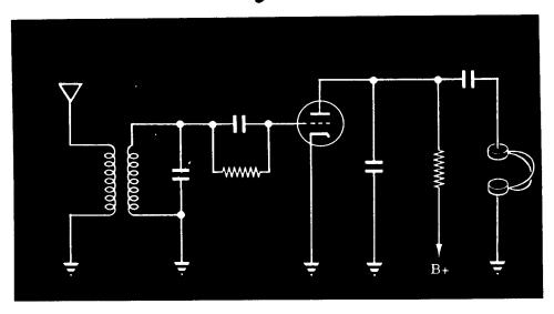
You will recall that the plate current of a triode is dependent upon the grid voltage. Consequently the audio frequency variations in bias should produce a corresponding pulsating plate current. Any radio frequency component of the plate current is filtered out by capacitors and RF chokes placed in the plate circuit. As a result, the voltage developed across the plate load is an amplified reproduction of the audio frequency voltage developed across the grid-leak resistor.
