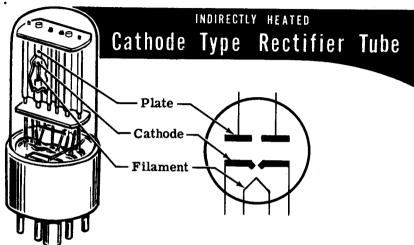
Vacuum tubes are constructed with a plug-in base which fits into a socket. The socket is permanently wired into the circuit and the tube is removable and easily replaced. Vacuum tubes have a relatively short life as compared to other components used in electronic equipment and a method of easy replacement is required.
