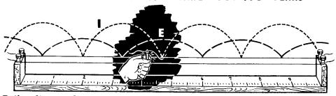
Both voltage and current peaks can be shown by using a long fluorescent light. The light areas are voltage peaks or current nulls.
