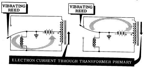
When the vibrator reed hits the lower contact, it puts a direct short across the electromagnet coil. This causes the magnetic field to collapse. Since the electromagnet can no longer hold the reed against the lower contact, the reed springs back past the center position and strikes the upper contact. When the reed strikes the upper contact, the following things happen.
