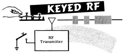
The simplest and most commonly used method of obtaining CW transmission is by "cathode keying." In this type of circuit, the key is connected in the cathode's DC return to ground. Thus, when the key is opened, no current can flow and no RF can be radiated from the antenna. When the key is closed, the circuit operates normally. The stage that is usually keyed in this manner is the master oscillator itself or the master oscillator plus one or more of the following amplifier stages.
