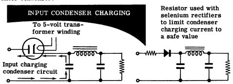
Because of the time lapse between pulses of direct current, the output of a half-wave rectifier requires more filtering than that of a full-wave rectifier and the filtered output voltage will be lower. Filter condensers used in half-wave power supplies are usually from 2 to 4 times as large as those used in full-wave power supplies. Increasing the size of the filter condensers provides additional filtering.
