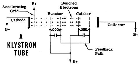
Then these bunched electrons reach the catcher grids and start the second tuned circuit oscillating. Since they keep arriving in bunches, they keep the second tuned circuit oscillating. The oscillations in the first tuned circuit will stop unless voltage is fed back from the catcher grids to keep it going. Of course the tuned circuits in the klystron are not coils and capacitors. They are cavity resonators.
