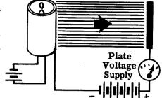
At this point, a further increase in plate voltage does not result in any additional current. The current does not increase because the cathode is emitting all the electrons it can. It is NOT normal to operate a diode at such a high plate voltage that changes in plate voltage do not produce changes in plate current.
