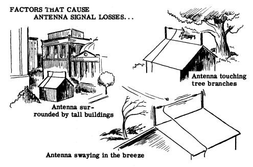
Signal losses will also be increased if a high resistance is present in the antenna circuit. To reduce resistance, all joints and connections should be carefully soldered and, wherever possible, the antenna and lead-in should consist of a single piece of wire with no joints.
