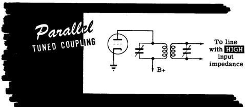
If the input impedance of the line is other than pure resistive, either of the above two tuned coupler circuits can be adjusted so that the reactance of the line is cancelled by the reactance of the tank circuit. This results in a pure resistive load, which is the requirement for maximum power transfer.
