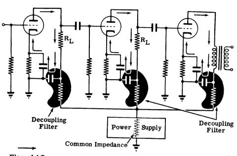
Flow of AC component of plate current
