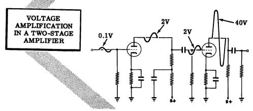
Suppose each amplifier stage can deliver an amplification of 20. If a 0.1 volt AC signal is applied to the grid of the first stage, the output of this stage will be  $20 \times 0.1 = 2V$ . Since the output of the first stage is connected to the input of the next stage there will be 2 volts AC on the grid of the second stage. The second stage amplifies the signal 20 times and produces an output voltage of  $20 \times 2 = 40V$ .
