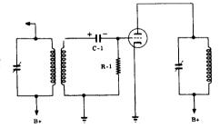
COMBINATION BIAS—A combination of fixed and grid-leak bias most commonly used in transmitters.
