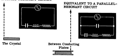
Taken by itself, the crystal acts like a series-resonant circuit. Together with its two plates, it acts like a parallel-resonant circuit. The frequency at which it vibrates depends on its thickness. Thick crystals vibrate slowly, thin crystals vibrate rapidly.
