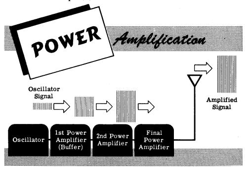
The RF signal is generated in the oscillator circuit and is amplified by the first and second power amplifiers which drive the final power amplifier. The powerful signal from the final power amplifier is fed to the antenna which radiates the signal into space.
