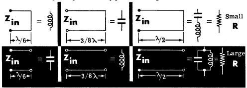
It is obvious from the above diagrams that the terminal conditions at the end of the line are the only factors which determine the type and magnitude of the input impedance at any point along the line.
