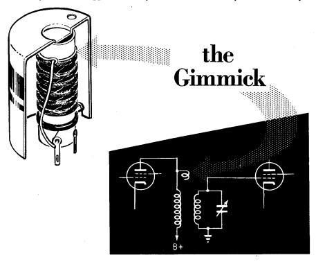
Perhaps you will recall some references, made in "RF Amplifiers," to the "Q" of a resonant circuit. This Q, which is equal numerically to the reactance of the coil divided by its resistance, determines both the selectivity and voltage gain that can be obtained from a resonant circuit. In order to keep the selectivity high, it is therefore necessary to use RF transformers whose resistance is fairly low.
