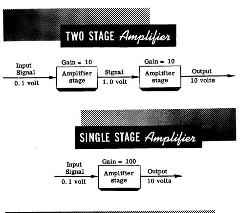
When an amplifier builds up the voltage 10 times, it has a voltage gain of 10. The voltage gain is the number of times a stage or group of stages amplifies the signal.
