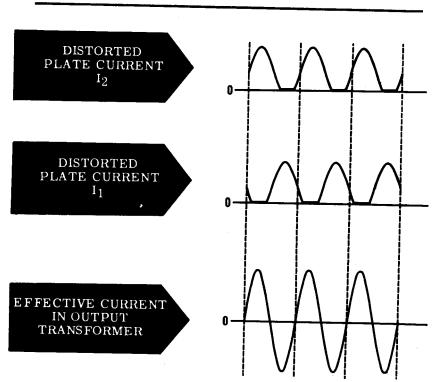
The reason that it is such a big advantage that the push-pull circuit reduces distortion is this—the tubes can be intentionally overdriven to produce a larger output and the output still will be practically undistorted.
