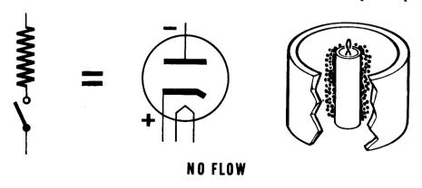
How Current Is Controlled in a Diode
