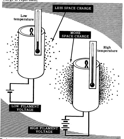
To increase the emission of electrons, you would have to raise the cath-ode's temperature by increasing the filament current. If, on the other hand, the cathode's temperature is lowered, the space charge will force some of its electrons to re-enter the cathode, resulting in decreased emission. The heater voltage for a tube is usually fixed. Various types of tubes operate with AC or DC heater voltages in the range from 1.25 to 117 volts.
