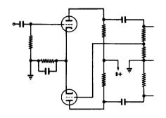
PUSH-PULL POWER AMPLIFIER — A circuit consisting of a voltage amplifier, a phase splitter (inverter), two power amplifier tubes and an output transformer.
