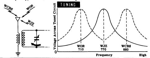
Changing Capacitor Setting—Changes Circuit's Resonant Frequency
