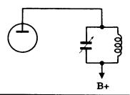
SHUNT FEED—A circuit arrangement in which the plate current of the tube flows through an RF choke and only RF voltage gets to the tank. This avoids the possibility of DC shock, but the RF choke cannot operate efficiently over a wide band of frequencies.
