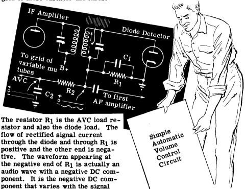
strength. The AVC filter circuit, consisting of  $R_2$ - $C_2$ , filters out the audio and  $C_2$  charges up to the negative DC component. It is this negative voltage that is applied through the AVC line to the grids of the variable-mu tubes in the preceding stages.
