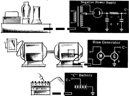
One of the advantages of fixed bias is that the tube remains cut off under no signal conditions.
