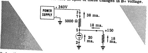
Under the operating conditions shown, 38 ma. flow through the dropping resistor, 20 ma. flow through the VR tube, and 18 ma. flow through the load. If the B+ voltage were to rise to +360 volts, the VR tube would have to adjust its internal resistance so that its plate voltage remained at 150 volts. Let's see if the VR tube is able to make this adjustment.
