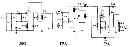
TUNING—For efficient operation, the plate tank circuit of the amplifiers must resonate at oscillator frequency. Adjusting the variable capacitor to reach this condition is called "tuning." Plate voltage is maximum and current minimum at signal frequency.
