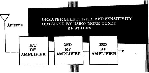
Since the RF amplifier stage is designed primarily for voltage amplification, any tube suitable for voltage amplification may be used. However, triodes are not considered satisfactory because they have a strong tendency to produce undesirable oscillations when employed in RF amplifier stages. Unless the triodes are carefully neutralized to prevent feedback, the oscillations produced are likely to cause considerable trouble.
