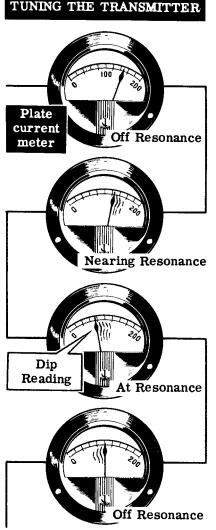
When the current is observed to be rising, the control should be turned in the opposite direction until it is set for minimum current. At this point, the tuned circuit is at the same frequency as the signal frequency and the output of the stage is maximum.
