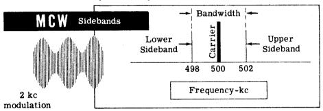
In a voice transmission, the modulating signal contains many frequencies—some as high as 5000 cycles per second. As a result, voice transmissions contain many sidebands (one sideband for each frequency) which may be as much as 5 kc above and 5 kc below the carrier frequency. This type of transmission, therefore, may cover a range of frequencies 10 kc wide.
