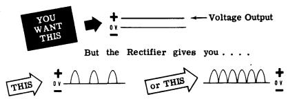
The job of the filter circuit is to smooth out the pulsations in the rectifier output and give you a steady voltage with little or no ripple. Filter circuits come in various forms, but all filter circuits are made up of various combinations of inductances and capacitors or resistances and capacitors. You will learn how these filter circuits work to smooth out the pulsations in the rectifier output as soon as you have done some work with various rectifier circuits.
