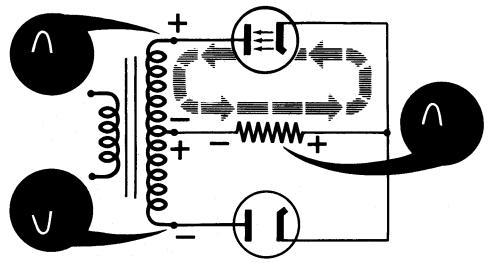
On the second half-cycle the plate of the upper diode is negative so that it cannot conduct, whereas the plate of the lower diode is positive so that current flows through it and through the load. Since both pulses of current through the load are in the same direction, a pulsating DC voltage now appears across the load. The full-wave rectifier has changed both halves of the AC input into a pulsating DC output.
