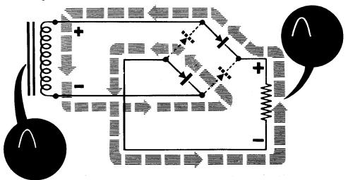
Then, when the AC voltage input swings negative, current flows through the other pair of dry metal rectifiers and the load. Notice that the current flow through the load is in the same direction during both half-cycles of the input wave. Therefore, the voltage developed across the load is pulsating DC which can, of course, be filtered just as any other pulsating DC output from a rectifier circuit.
