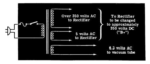
How a Power Supply Works-The Rectifier
