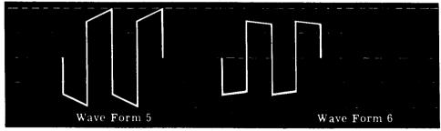
You will notice that the new input wave form (no. 4) is smaller than wave form 1, the old input. This is so because the voltage that was fed back is out of phase with, and so subtracts from, the original signal input. Thus the output is smaller than it would ordinarily be and the gain of the stage is apparently lessened. More important than the loss of gain is the decrease in the amount of distortion. This method of decreasing distortion is known as "degeneration" or as "negative feedback."
