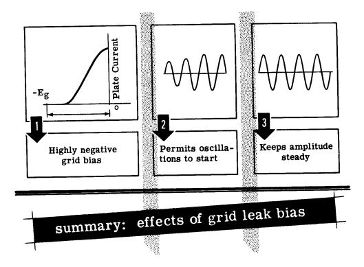
Grid leak bias has one disadvantage. If oscillations should cease, even momentarily, the high negative grid bias would be lost. A large flow of electrons from cathode to plate would occur. This average plate current flow would be so large as to damage or ruin the vacuum tube.
