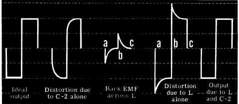
To improve the steepness of the steep portion of the square wave, an inductance (L) is placed in series with the plate load resistor (R-1). The back emf set up in this inductance every time the plate current changes will be in such a direction as to cause a peak to appear in the plate voltage.
