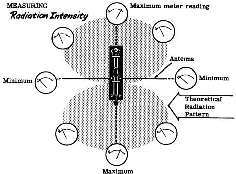
To show that movement of objects near the antenna affect the radiation pattern, the instructor sets the wavemeter down at a given point and walks between the meter and the antenna. Observe that the meter reading varies sharply as the instructor walks about.
