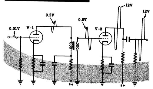
The voltage across the secondary of the transformer (0.6V) is now applied to the grid of V-2. If we assume that the gain of V-2 is equal to  $\mu$ , then V-2 will amplify this signal 20 times. Therefore, the output voltage at the plate of V-2 will be—20 x 0.6 = 12V.
