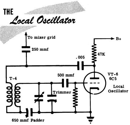
Now that you have seen the complete schematic of a superhet, it will be worth your while to spend a little time analyzing the function of the circuit components used in the oscillator, the mixer, and the detector stages.
