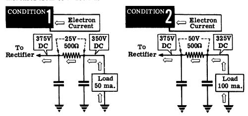
Similarly a change of 100 ma. in the load current will cause the B+ voltage to drop 50 volts. Such a rise and fall in output voltage is very undesirable in electronic equipment. Voltage regulator circuits might be added to compensate for this voltage change due to the filter resistor, but it would require a large and expensive circuit to compensate for changes such as are indicated here.
