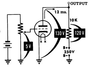
the voltage on the plate is now only 130 volts—a decrease of 70V. Note that the sum of these two voltages still adds up to the B+ voltage of 250V. Thus, a change of only 5 volts on the grid has changed the plate voltage 70 volts—an amplification of 14 times.
