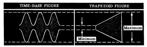
The two 'scope presentations shown above are for the same condition of modulation. You could determine the maximum height (peak) and the minimum height (trough or valley) of the RF from either figure. You could also determine the linearity of the modulation from either presentation, but it is easier to do so from the trapezoid.
