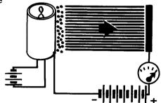
If we had reduced the filament voltage, the current would have decreased because the cathode could not emit as many electrons as before. In practice, the filament voltage is not varied. Changes in plate current are achieved by varying the plate voltage as already described. However, after a tube has been used for some time, the cathode's emission decreases and the result is the same as if the filament voltage were decreased.
