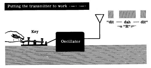
A signal of this type contains intelligence since a message can be obtained from it. The radio would produce a sound somewhat like "dit-dah-dit" which a radio operator understands as the letter "R."
