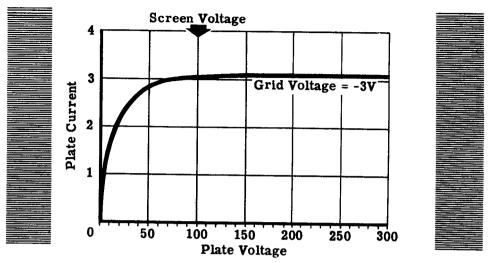
Curve No. 1: Over a wide range of plate voltages, the pentode plate current does not vary. But this is not saturation; in the next curve you will see that it is possible to draw more current than this. The reason the current doesn't vary over this range of values is that the screen shields the plate from the cathode's space charge.
