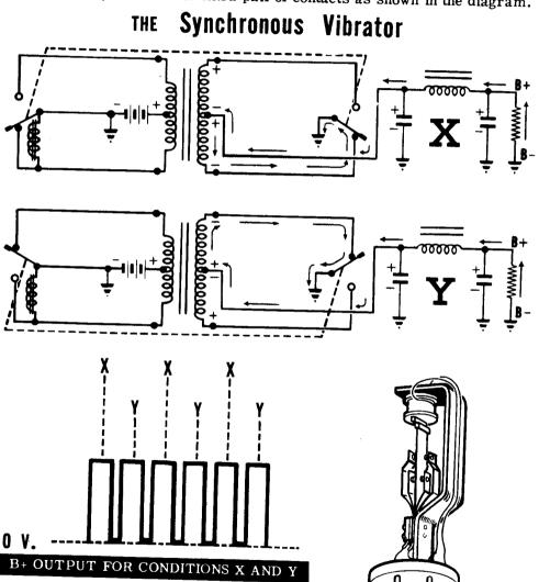
The two vibrating reeds shown connected together by the dotted line in the diagram are actually one reed placed between two pairs of contacts. The action of the reed between the transformer secondary contacts produces the same results as a full-wave rectifier. RF chokes and buffer condensers are used in this vibrator circuit in the same manner as in the non-synchronous vibrator to eliminate contact sparking and radio interference.
