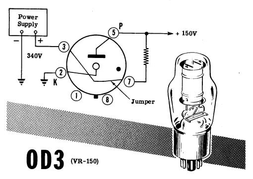
Notice that there is a "jumper connection" between pins 3 and 7 inside the tube. If pins 3 and 7 are wired in series with the circuit, this jumper will act as a switch. When the VR tube is pulled out, the circuit requiring the 150 volts will be disconnected from the power supply. If this jumper were not connected as a switch and the VR tube were pulled out, the 150 volt circuit would receive more than 150 volts-resulting in damage to its components or in improper operation.
