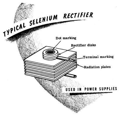
A perfect rectifier would offer no resistance to current flow in one direction and infinite resistance in the opposite direction, but such a rectifier is only theoretical. Practical rectifiers used in power supplies actually have low resistance in one direction and very high resistance in the opposite direction. For dry metal rectifiers these resistances can be measured with an ohmmeter.
