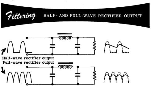
The higher the frequency of the AC input voltage to a power supply the lower the value of the filter condensers required. The time between pulses is shorter at higher frequencies and the inductive action of the choke is greater at higher frequencies.
