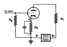
TRIODE AMPLIFIER OPERATION — The variation in voltage output (plate voltage) of a triode, used as an amplifier, may be ten or more times larger than the variation in the grid voltage (AC signal).
