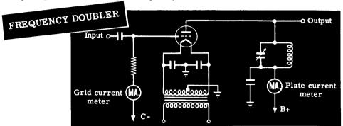
The circuit of a frequency doubler appears to be the same as that of an amplifier which operates at the input frequency. The only differences are that the plate circuit will be tuned to twice the input frequency and no neutralization is required since the input and output operate at different frequencies. This reduces the possibility of self-excited oscillations.
