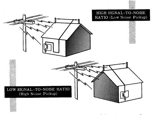
The second method is by increasing the height of the antenna as much as practical considerations will allow. This tends to increase the signal strength and reduce the amount of noise.
