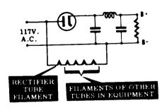
volts B+ from a 117-volt AC power line without the use of a transformer. The circuit consists of two half-wave rectifiers and two capacitors. The capacitors are connected in series and each is charged up to peak line voltage resulting in the voltage doubling effect. The filaments of the rectifier tube and the other tubes in the circuit are all
