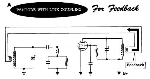
With sufficient coupling, feedback energy will compensate for resistance loss in the grid tank and oscillation will continue.
