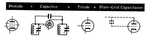
Thus you can see that feedback to sustain oscillation can be accomplished without the use of coil or capacitor. The internal capacitance of tube elements provides the feedback.
