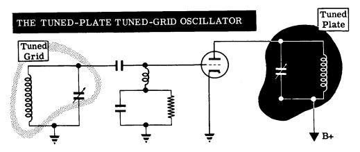
Feedback is accomplished without using either capacitor or coil to couple the energy back. To prove this, suppose you start with the above circuit, but with a pentode tube in place of a triode and use link coupling to feed back energy from plate to grid tuned circuit.
