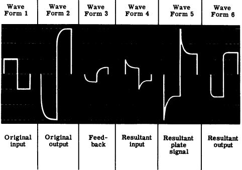
The important thing to remember is that the signal which is fed back contains the distortion that exists in the output. When this signal is combined with the original grid signal, the distortion appears "backward." The resulting plate signal has distortion that is opposite to the distortion originally existing in the output. In this respect, negative feedback does almost the same thing as a compensating network. The important differences are these:
