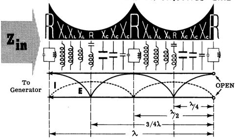
The following diagrams illustrate different lengths of open and shorted lines and the input impedance they present to a generator.
