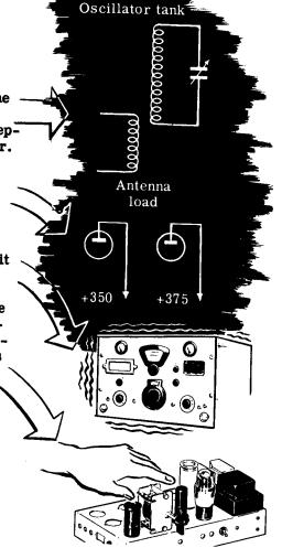
The importance of maintaining a stable frequency becomes apparent when you realize that most transmitting stations operate at one fixed frequency. At times it is essential that transmitter and receiver maintain constant twenty-four hour communications relations. If the frequency shifted, vital messages or parts of them might never be received.
