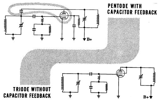
The pentode with capacitor feedback will support oscillation. The triode without capacitor feedback will support oscillation because it, too, provides feedback: not through an outside capacitor but through the capacitance between the plate and the grid of the triode. The pentode has such a low plate-grid electrode capacitance that an added capacitor is needed. The triode has more plate-grid capacitance and doesn't require an added capacitor. Both employ capacitance feedback.
