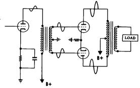
DISTORTED WAVE FORMS due to overdriving the tubes do not noticeably affect the current wave form in the output transformer of a push-pull amplifier.
