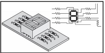
The "8" LED display is mounted on a board and to prevent burning out the display with excess current, permanent resistors have been wired in.
