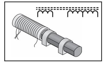
**Transformer:** Did you know that if you were to wrap two wires from different circuits around different ends of an iron bar, and if you were to add current in the first circuit, it will magnetically create current in the second circuit? That's exactly what a transformer is! Transformers are used to isolate parts of a circuit, to keep them from interfering with each other.
