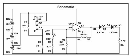
and press the key. The LEDs light brightly. Calculating the output voltage gives  $1.5V \times ((220k\Omega / 32k\Omega) + 1) = 11.8V$ . However, the actual output voltage will be limited by the available battery voltage, which is 1.5V + 3.0V + 3.0V = 7.5V.
