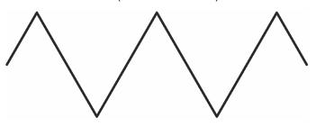
The shape of this wave results from the slow charging of the  $0.1\mu$ F capacitor through the control and the  $100k\Omega$  resistor, and the capacitor's discharge through the PNP and NPN transistors.
